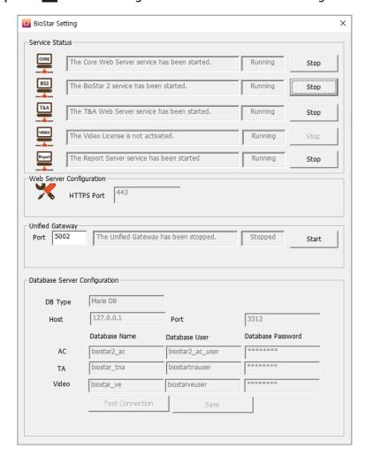
**2** Click the **Stop** button for all BioStar 2 services. **Database Server Configuration** is activated.
